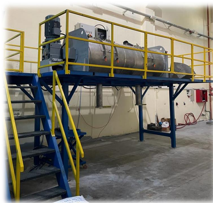
2000 TONS CAPACITY RESIN MIXING AND CURING BOILER
